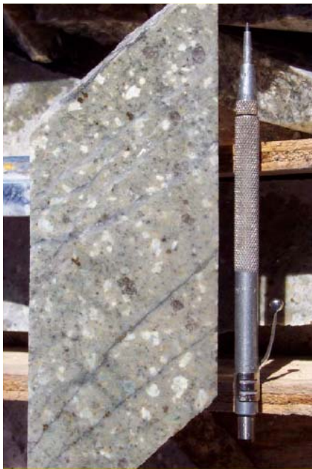
Figure 5: Gold-bearing porphyritic dyke, Donlin Creek Gold Deposit.
