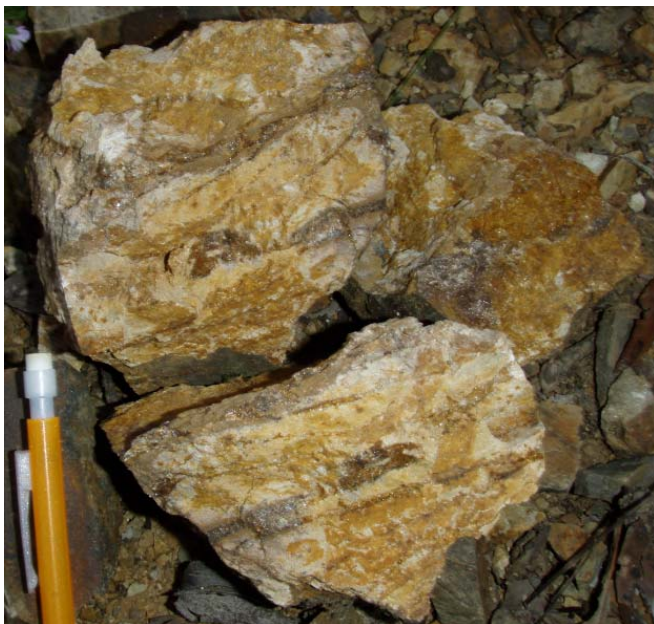
Figure 7: Hudsons McCrossins Sample S177B (0.46 g/t gold). Narrow, close-spaced, sheeted ferruginous quartz veins in metasediments.
