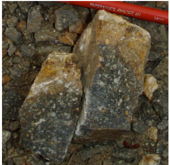
Figure 6: Shaft H1 (see Figure 1) excavated in a porphyritic dyke exhibiting pronounced limonite staining after oxidised sheeted sulphide veins and disseminated mineralisation.
