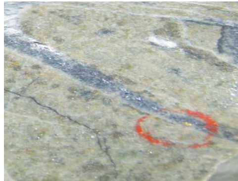
Martins Shaft – Sample SGRDD002 – 36.80m. Free gold (around 1mm long) in quartz-antimony-arsenopyrite-carbonate vein.
