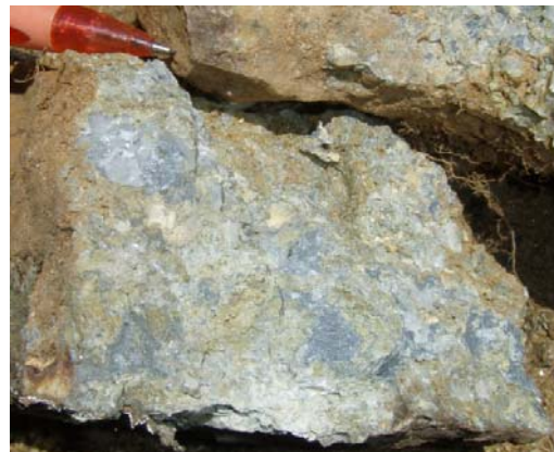
Frasers Find – Sample FF5B – High grade quartz-sulphide (abundant arsenopyrite, pyrite, galena) from the dump by the main shaft, assayed 76.9 g/t gold (2.47 ounces), 287 g/t silver (9.23 ounces) and 1.78% lead/tonne (ALS Certificate of Analysis BR12004879).
