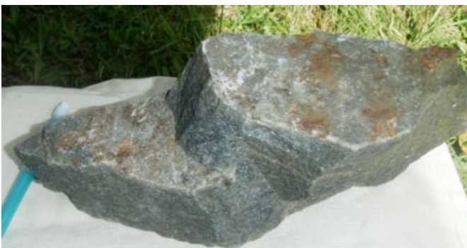
Melvaines Mine, Sample MM1, 2.12 grams/tonne Gold. Narrow sheeted quartz-sulphide veins in altered dyke like those drilled at Martins Shaft.
