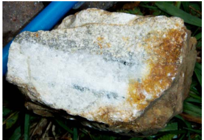
Melvaines Mine, Sample S414, 13.75 grams/tonne Gold, 2cm wide sheeted quartz-sulphide vein in quartz-sericite altered dyke.
