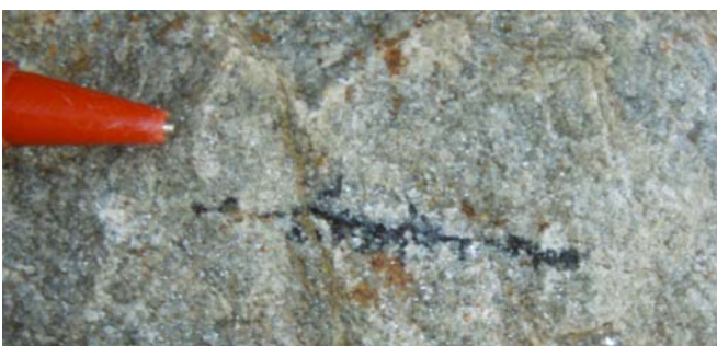
Melvaines Mines, mirolitic textures with tourmaline (black mineral), a classic diagnostic IRGS characteristic. Indicative of the late stage volatile portion of the magma becoming trapped within the body of the dyke. The last magmatic stages are frequently associated with gold deposition in IRGS. This is clearly the case at Melvaines Mine.
