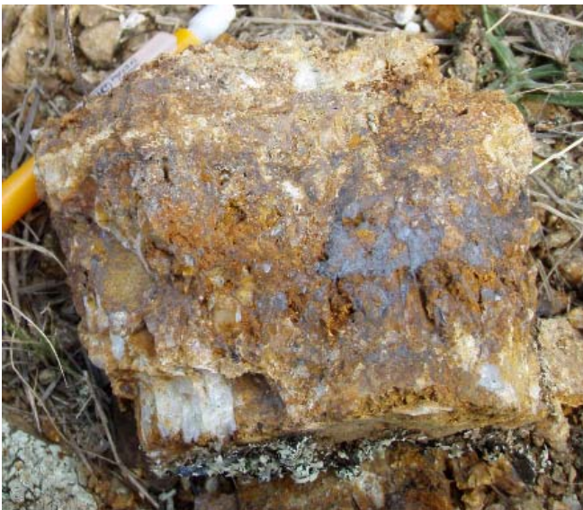
Sample S217: Ferruginous, vuggy, close-spaced (1-2 centimetre spacing) comb quartz veins (epizonal character) up to 20mm wide. Assayed 2.0 g/t gold, 3.54 ounces/t silver and 0.78% lead/t.
