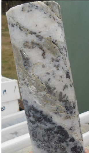
Figure 11: SGRDD004 from 58-59m, 19.6 grams/tonne gold, 67.8 grams/tonne silver, 0.64% antimony (Sb); (HQ core, diameter 63.5mm).
