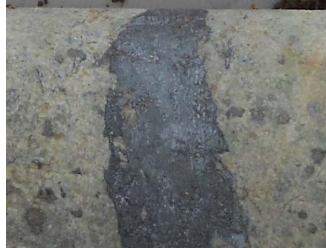
Figure 12: SGRDD004, antimony sulphide vein, 30mm wide, in phyllic altered felsic dyke (around 60m); (HQ core, diameter 63.5mm).
