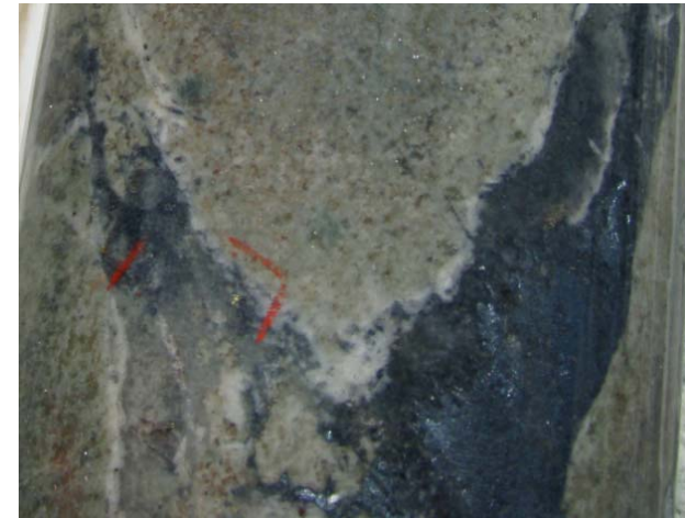
Figure 8: Visible gold in core SGRDD002. Visible gold (1 mm x 1mm, red lines right-hand-side) in sheeted, antimony-quartz-carbonate veins, (around 36.0m; 35-36m, 15.2 grams/tonne gold); (HQ core, diameter 63.5mm).
