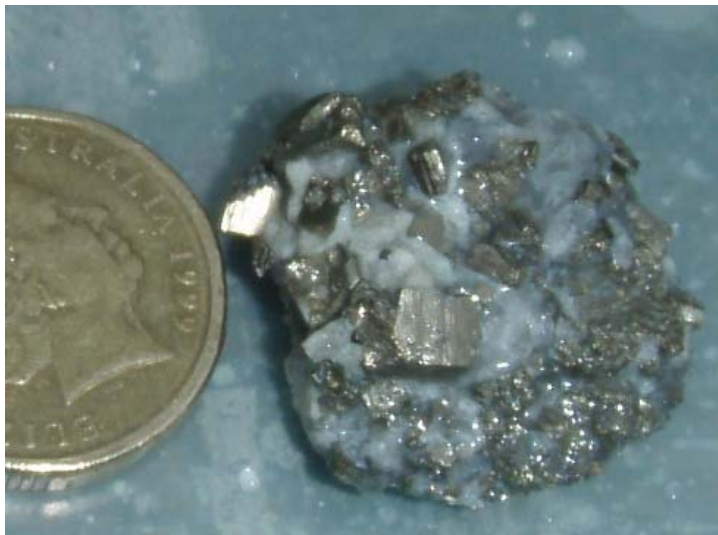
Figure 13: SGRR0011, euhedral pyrite, 1.53 grams/tonne gold, 60-61m.
