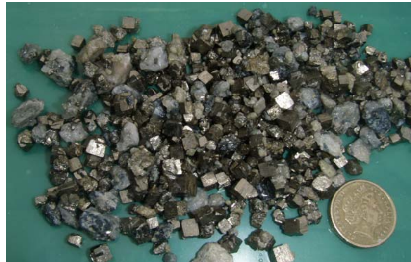
Figure 14: SGRR0017, euhedral pyrite and arsenopyrite, 86-89m.
