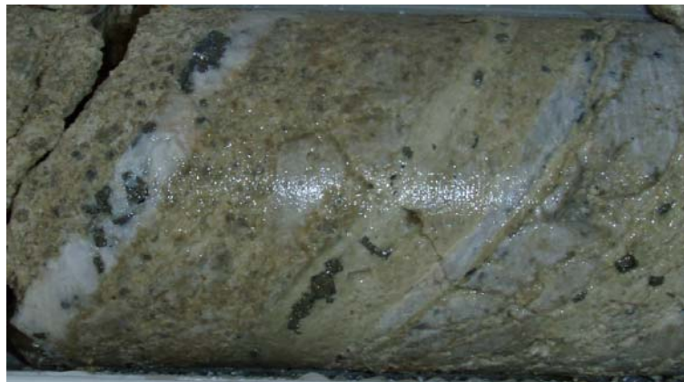
Figure 9: SGRDD002, close-spaced sheeted, carbonate-quartz-pyrite-arsenopyrite veins in phyllic altered felsic dyke (around 27m). 27-28m, 10.5 grams/tonne gold, 13.35 grams/tonne silver (HQ core, diameter 63.5mm).
