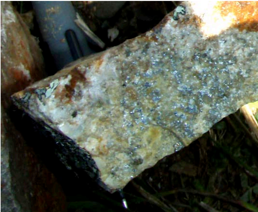
Site RE6, (56 J 354662mE 6619920mN), sheeted vein in felsic dyke exhibiting sericite- abundant sulphide (arsenopyrite) alteration – Martins Shaft-style mineralisation.
