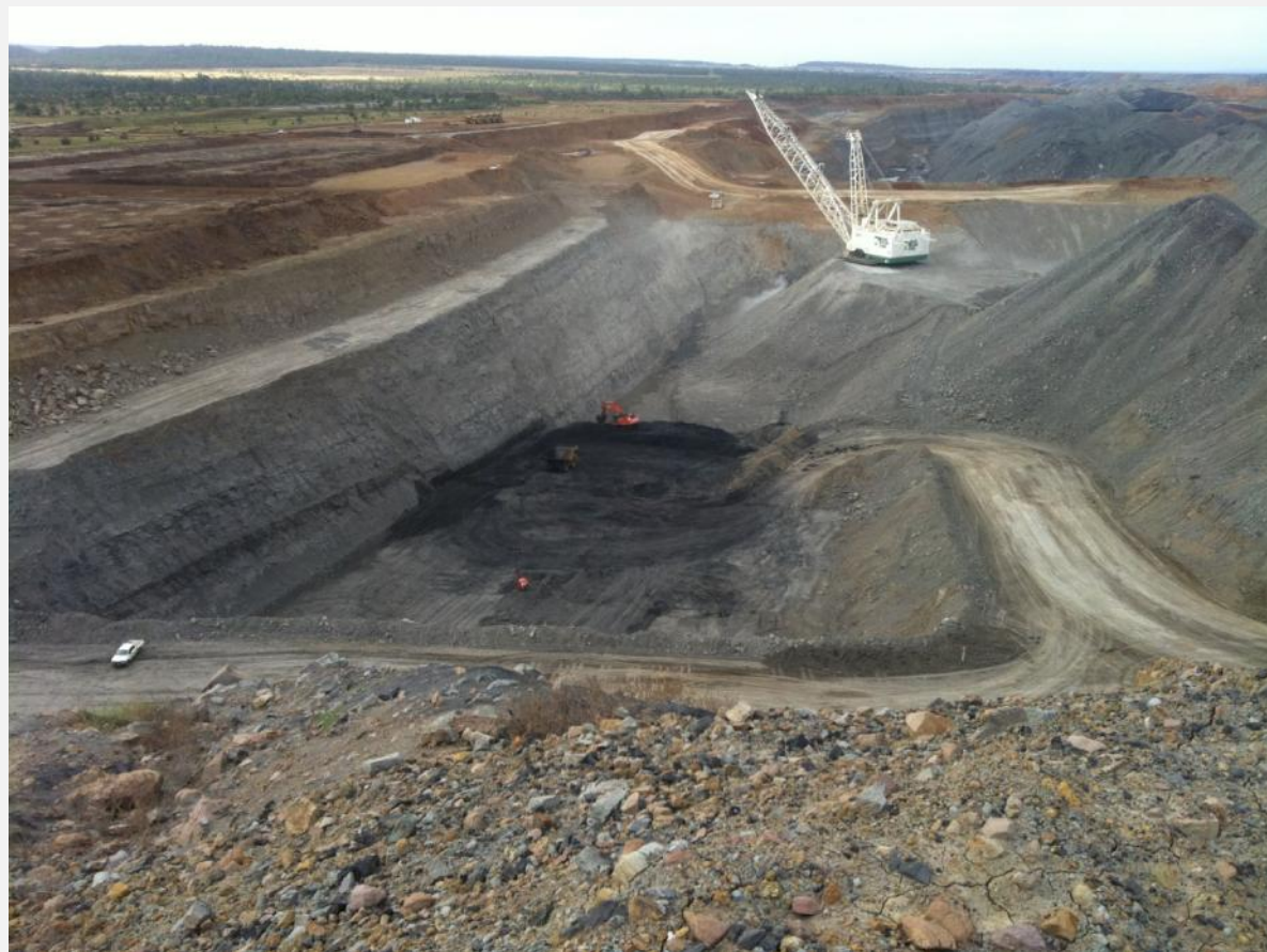
Isaac Plains dragline on overburden with coal excavators on pit floor
