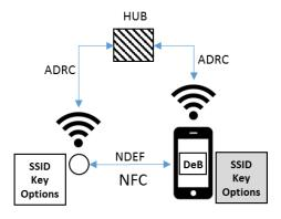
Figure 6 – On-boarding IP-based IoT devices
