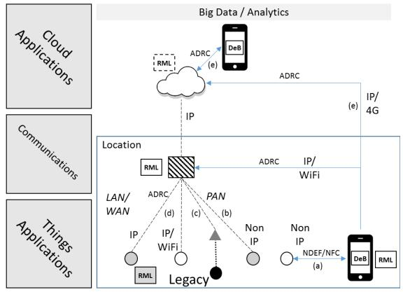
4(b)). The hub will have been placed in a location so that a personal area network (PAN) connection to the "thing" is possible. The hub will also have a copy of the RML file as a result of the on-boarding process. Control can then occur via the ADRC protocol from smart device to the "thing" using a local fixed or wireless IP network.
