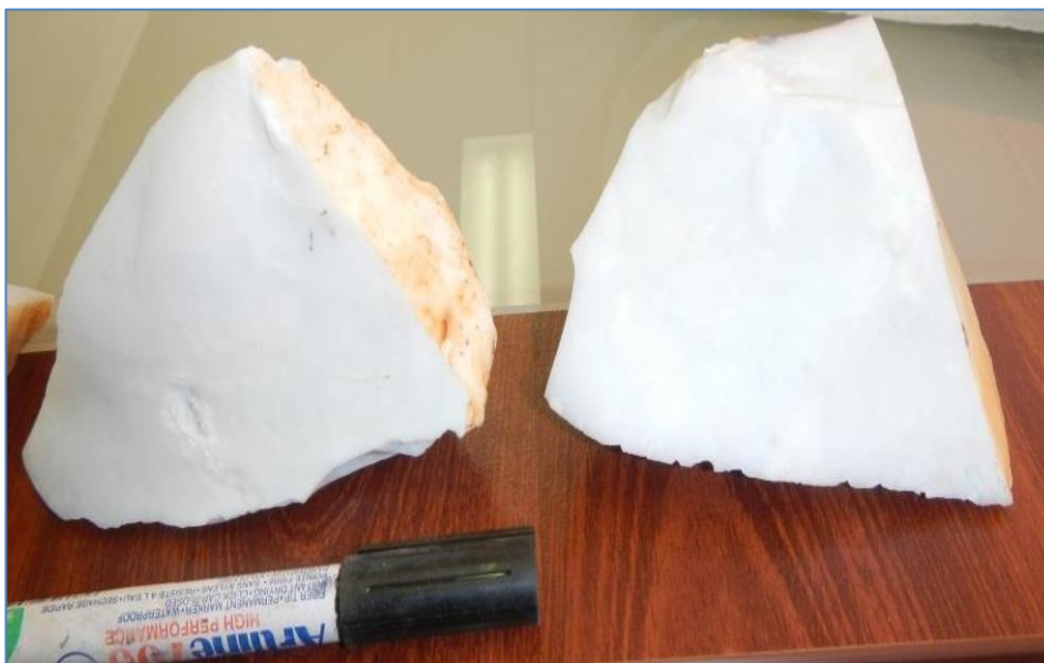
Figure 2. Visually-selected Dingo Hole Silica from outcrop.
