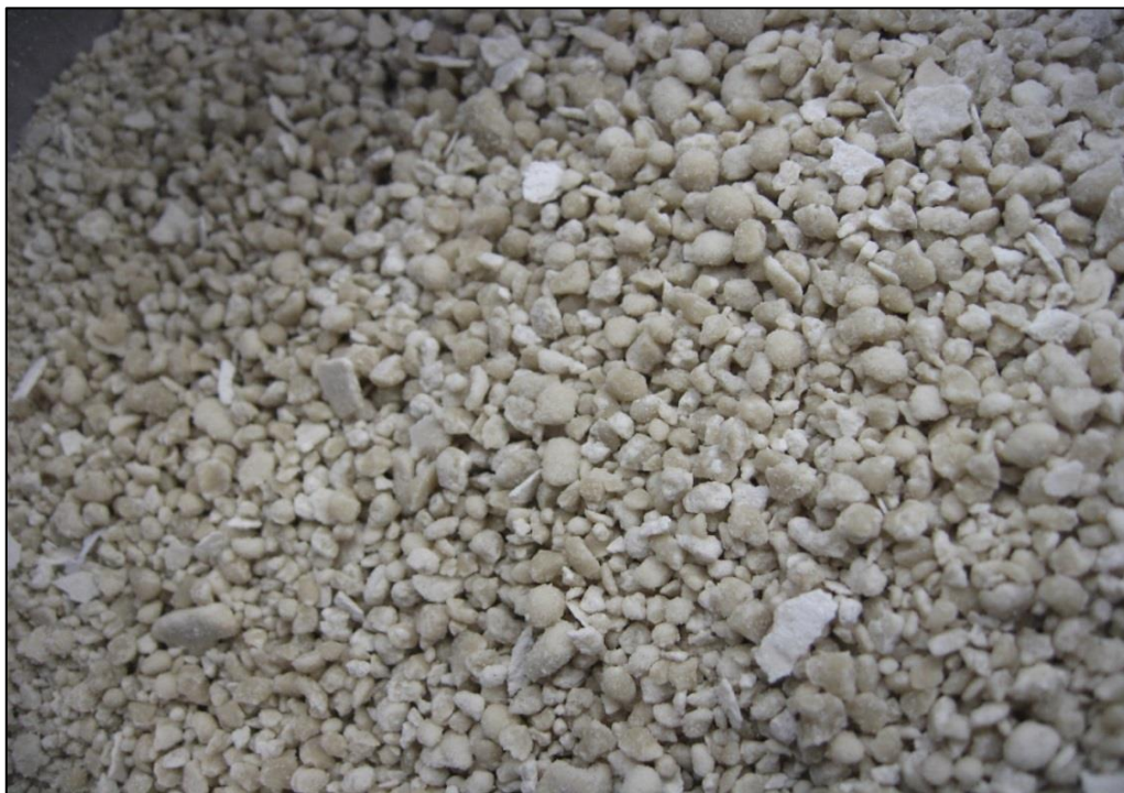
Figure 6. Di-Ammonium Phosphate fertiliser produced from Ammaroo phosphate rock at Prayon's laboratory.
