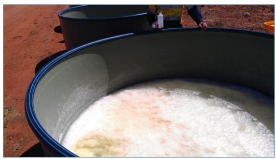
Figure 2. Recent picture at Karinga highlights the amount of salt and potassic-rich bittern remaining after months of evaporation in a single tank. The bittern is now removed so that it may be crystallised for processing of potassium magnesium sulfate and other compounds.
