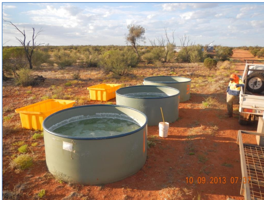
Figure 6. Evaporation trial progress as of 10 September. Note the ring of halite around the rim and the rafts of halite nucleating on the brine surface.
