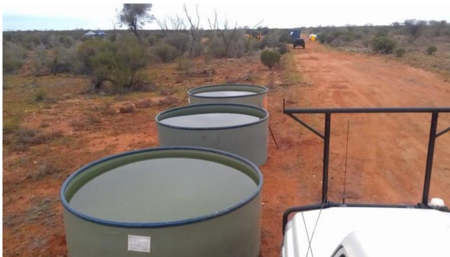
Figure 6. Evaporation tanks with 12,000 litres of brine at start of trial
