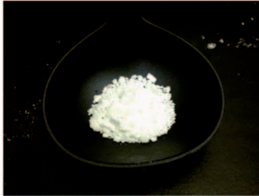
Figure 6: Mixed dry salts uncrushed produced from evaporation prior to flotation.
