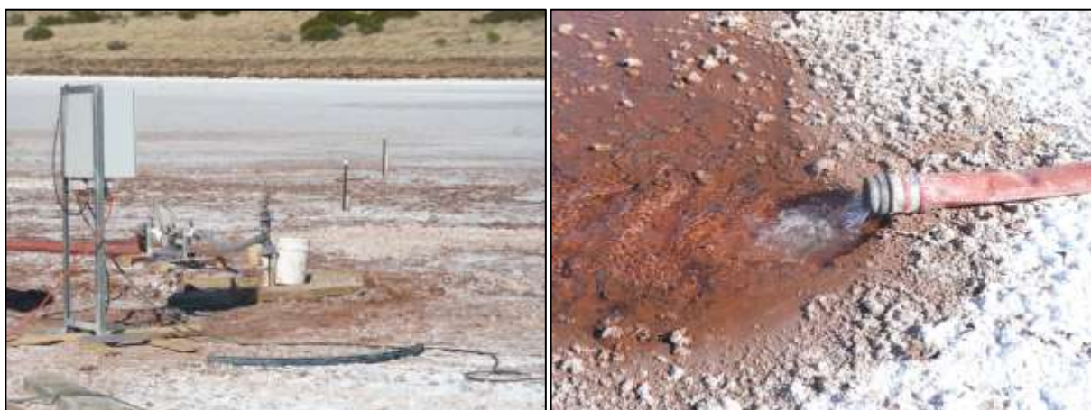
Figure 8: Pump testing of bore hole at Karinga Creek.
