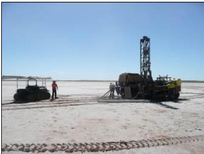
Figure 7: Aircore drilling at Karinga Creek Potash project.
