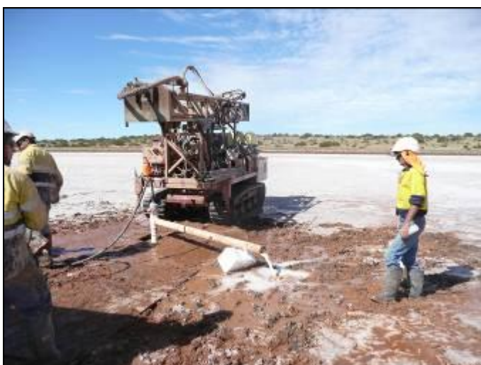
Figure 8: Flow testing of bores.
