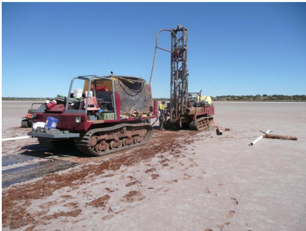
Figure 8: Tracked air core drill rig and compressor support truck driven onto the lake edge on mats
