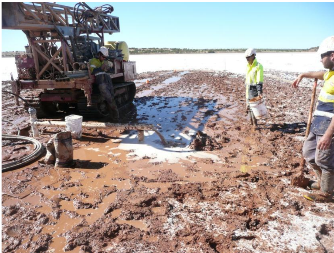
Figure 10: Flow testing a bore from 3 m depth on Murphys Lake
