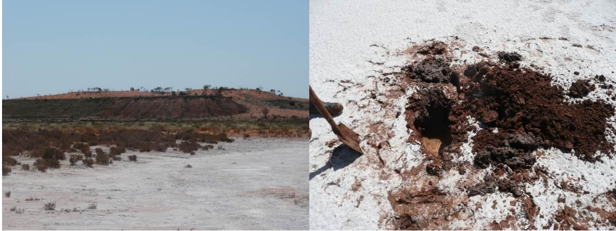
Figure 5. Typical clayey sands and gypsum rich lake bed sediments
