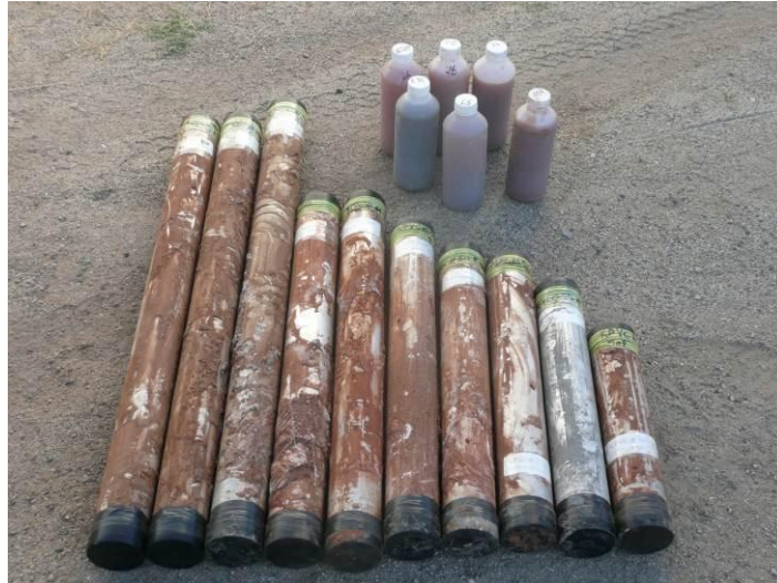
Figure 2. Vibracore drill core samples in sealed tubes and corresponding brine samples
