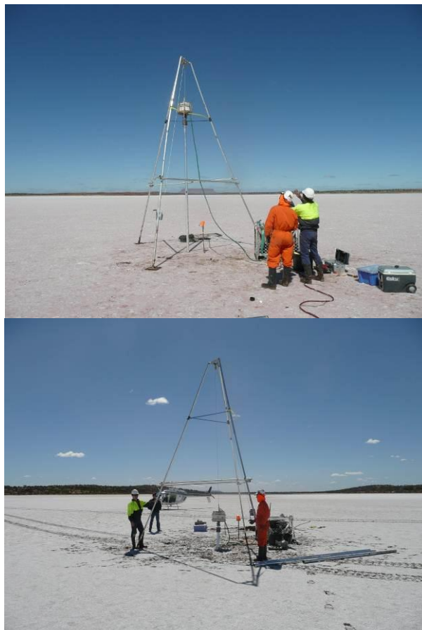
Figure 1. Vibracore drilling at Karinga Creek
