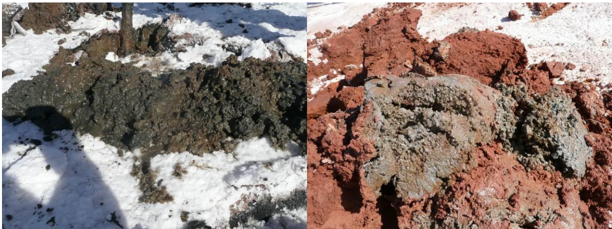
Figure 5. Typical clayey sands and gypsum rich lake bed sediments
