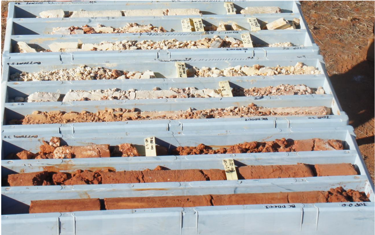
Figure 2: PQ Diamond Drill Core DDH 3 showing red surface sand and loam to 3 metres with 6 metres of phosphate bed immediately beneath. Each tray length is one metre. The highest grade white/yellow phosphate up to 32% P 2 O 5 occurs from 5 to 9 metres below surface.
