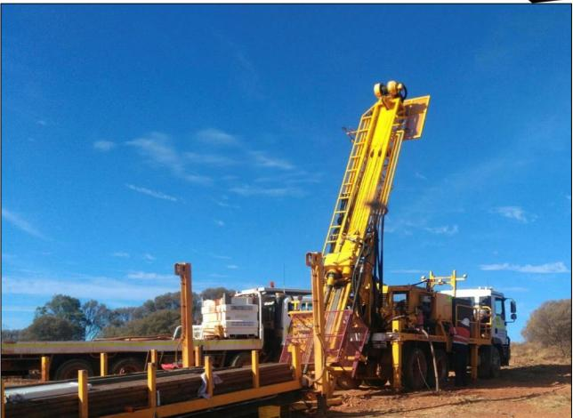
Image 1. Diamond Core Drill Rig operating at the Earaheedy Project
