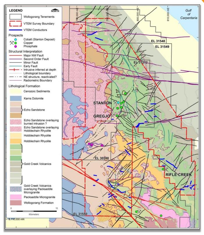
Figure 10 VTEM conductor picks overlying new litho-structural interpretation. (VTEM in Blue - not ranked by colour)
