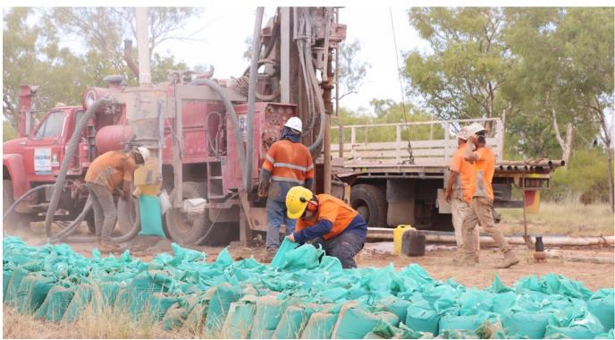
Figure 1 RC Drilling rig Benmara Project September-October 2021 - local NT based contractor Geo Drilling
