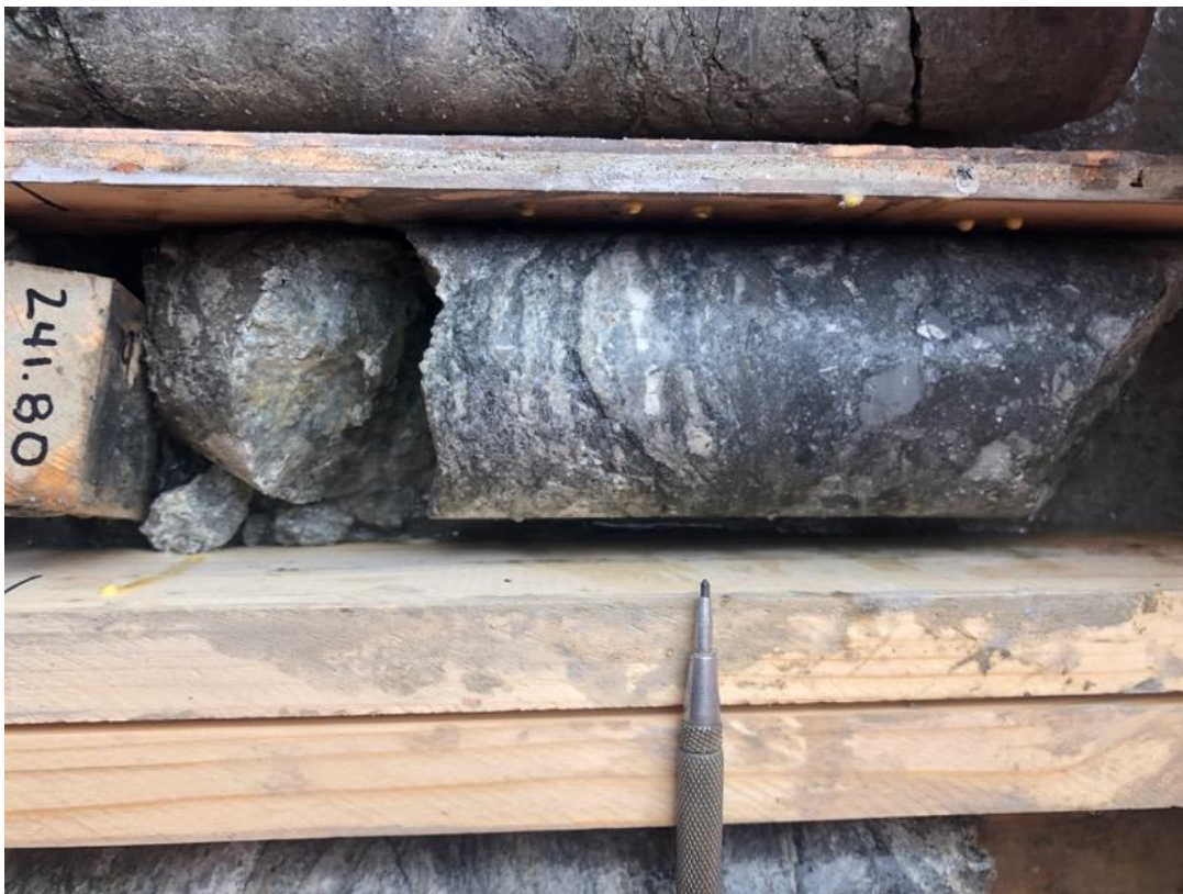
Figure 4. Hole ID 20AU001; brecciated vein with abundant arsenopyrite in paragneiss at 241.80m depth.
