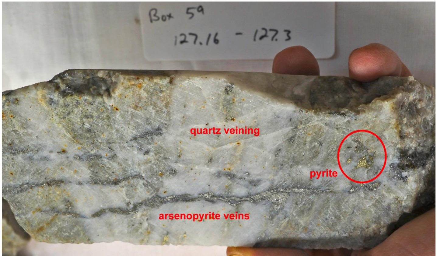
Figure 2. Hole ID 20AU001; cut ½ drill core 127.16m to 127.3m quartz veins, arsenopyrite, pyrite in paragneiss.
