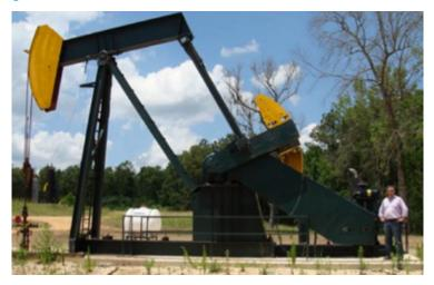
Typical pumping unit on a Four Rivers well
