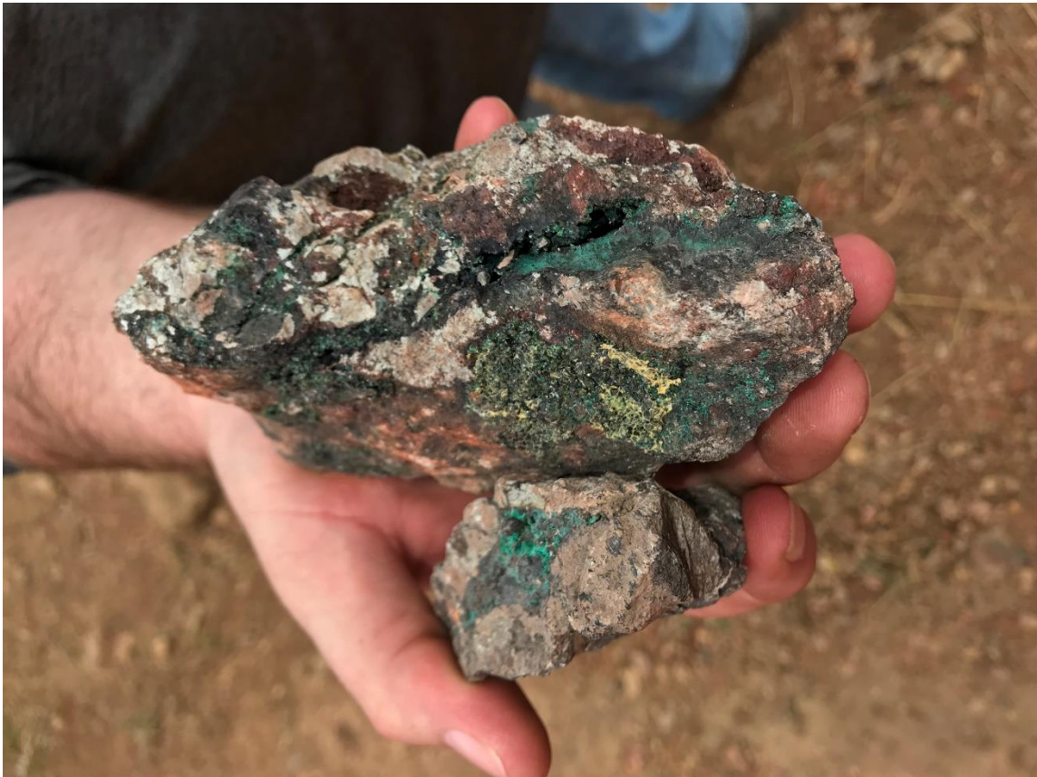
Figure 3. Copper-cobalt (malachite & heterogenite) mineralisation from the north eastern end of the Tombolo anticline. Sporadic mineralisation is mapped for some 1.5 km along the contact between the Mines Series and Nguba Groups
