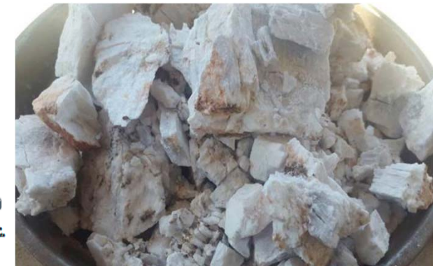
β-spodumene – post decrepitation of spodumene & petalite
