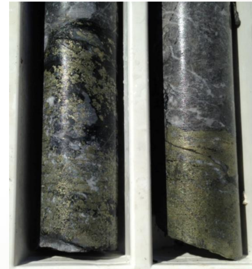
Drill core CCD03 – semi-massive chalcopyrite bands. Contain only minor pyrite
