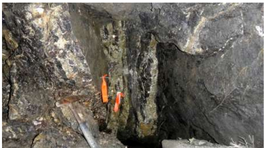
Photos taken during underground channel sampling. Left: channel made after sampling of pyrite and quartz dominated mineralisation. Above: Both phases of mineralisation visible – to left of orange tape, sphalerite, pyrite, quartz and carbonate to the right pyrite and quartz
