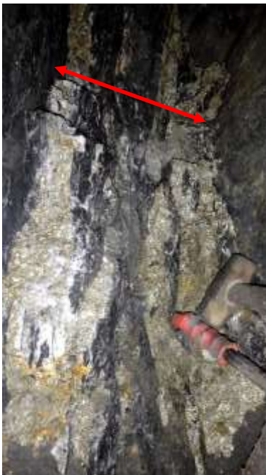
Photos taken during underground channel sampling. Left: channel made after sampling of pyrite and quartz dominated mineralisation. Above: Both phases of mineralisation visible – to left of orange tape, sphalerite, pyrite, quartz and carbonate to the right pyrite and quartz
