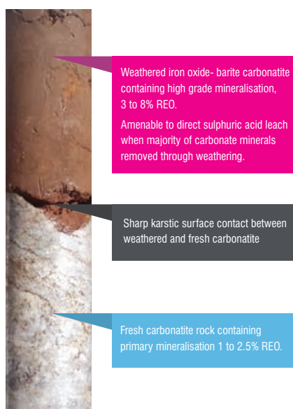
▲ Figure 5: The sharp contact between the weathered (brown) and fresh carbonatite (white) in the Bastnaesite Zone.
