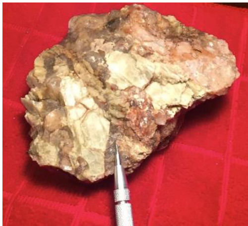
Figure 6: Photograph of Coarse grained spodumene from the SG pegmatite.
