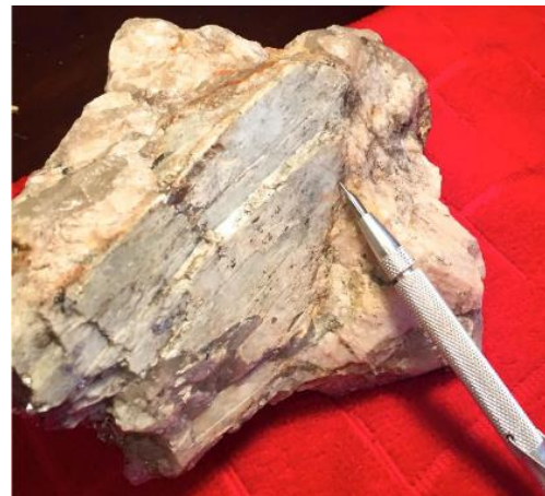
Figure 7: Photograph of Coarse grained spodumene from the new pegmatite.
