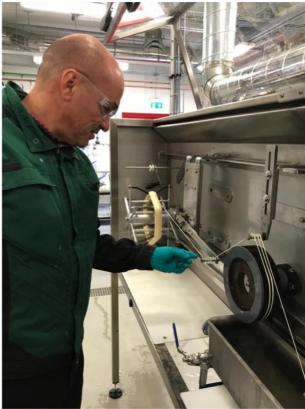
Nullarbor fibre going through the spinning process using standard industrial equipment.
