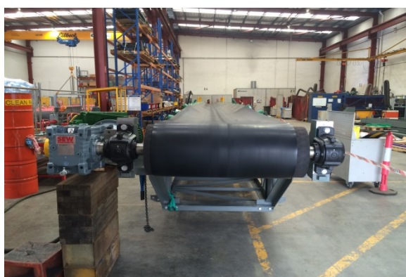
Figure 4: MFU conveyor ready for transport to site
