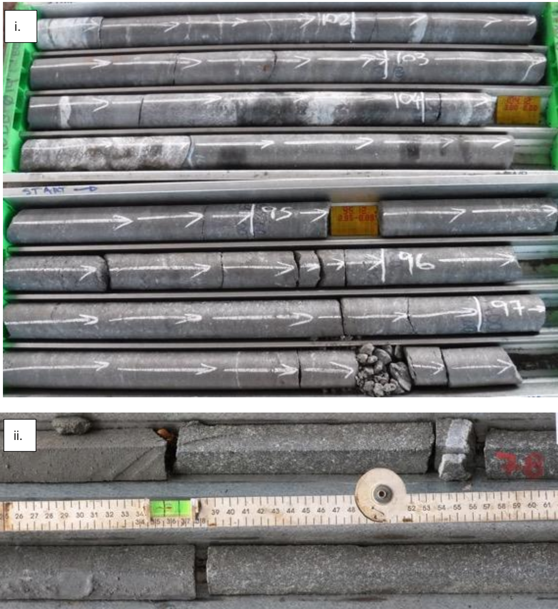
Figure 3. Graphite samples from MODD0010 on 5873L. (i.) Box 35 (top) and Box 33 (bottom). (ii.) quartered graphitic schist from Box 28
