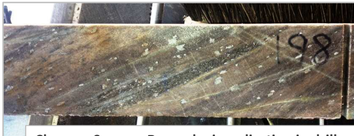
Close up Spargos Reward mineralisation in drill core
