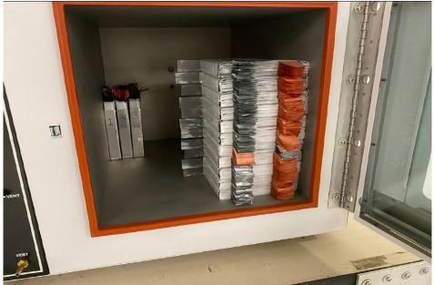
Figure 3: Production cells drying out ahead of cell assembly and testing
