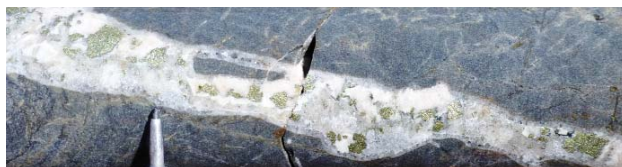
Figure 3: Quartz +calcite +chalcopyrite vein at 203 m in hole OS13D02 representing part of 1 m interval (202-203 m) assaying 0.49% Cu.
