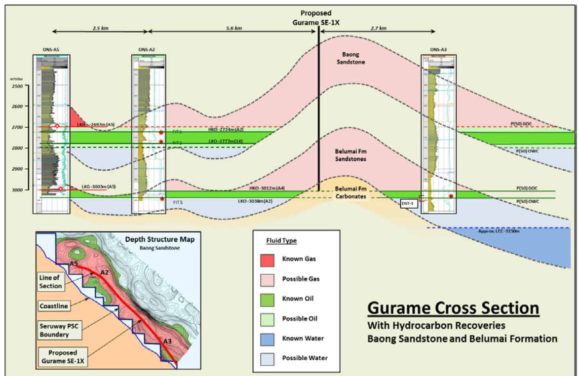
Gurame SE-1X has been located to intersect the prospective deep reservoir section structurally up dip from existing well control, near the crest of the closed structure which has been defined by modern 3D seismic data. A major objective of the well is to determine the performance capability of the Baong and Belumai reservoirs. Drilling techniques will be optimised to limit formation damage.
