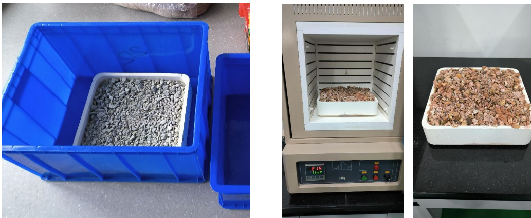
Figure 3 – Calcination of Spodumene – Before and After
