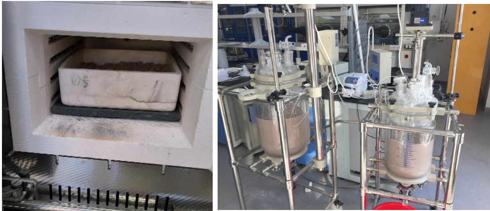
Figure 4 – Sulphation Roasting (L) and Leaching (R)
