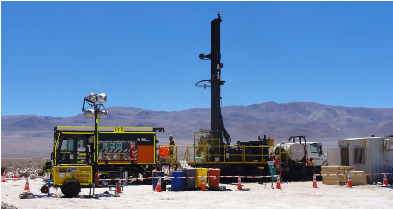
Figure 2: Sonic drilling rig setting up on one of the drill sites
