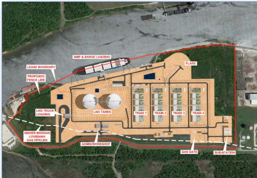
Proposed Site Layout for the 8 mtpa Magnolia LNG Project
