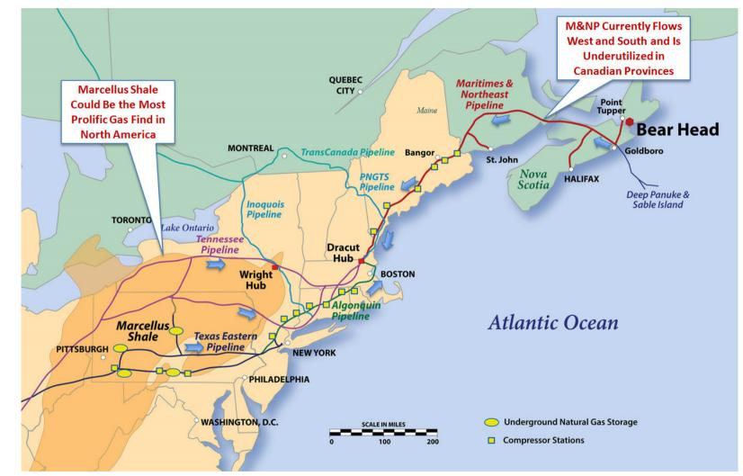
Gas Supply to the Bear Head LNG Project requires the construction of a gas transmission pipeline off the M&NP pipeline to deliver gas from Goldboro to the Bear Head LNG terminal site
