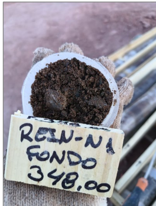
Figure 2. Diamond drilling rig at platform K23 and a representative gravelly sand from K23D40 at 348 m bgs
