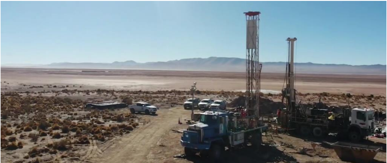
Figure 2: Foraco diamond drill rig (right) and rotary rig at Cauchari overlooking the Cauchari salt lake and development of the adjoining pre-production areas of Ganfeng / Lithium Americas.
