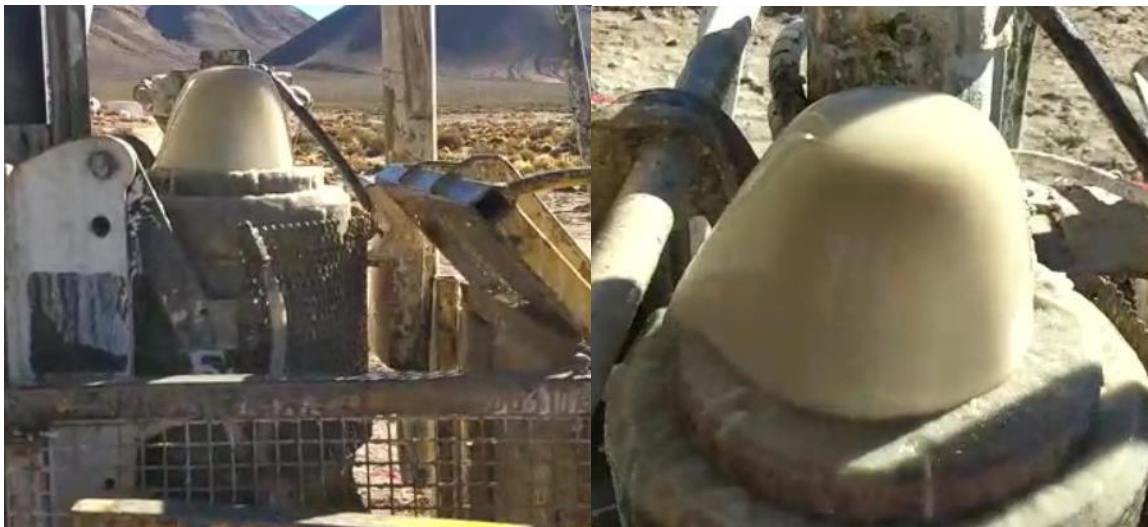
Figure 3: Lithium bearing brines flowing out of the drill head (pale yellow upside down cup shape) from high pressure horizons
