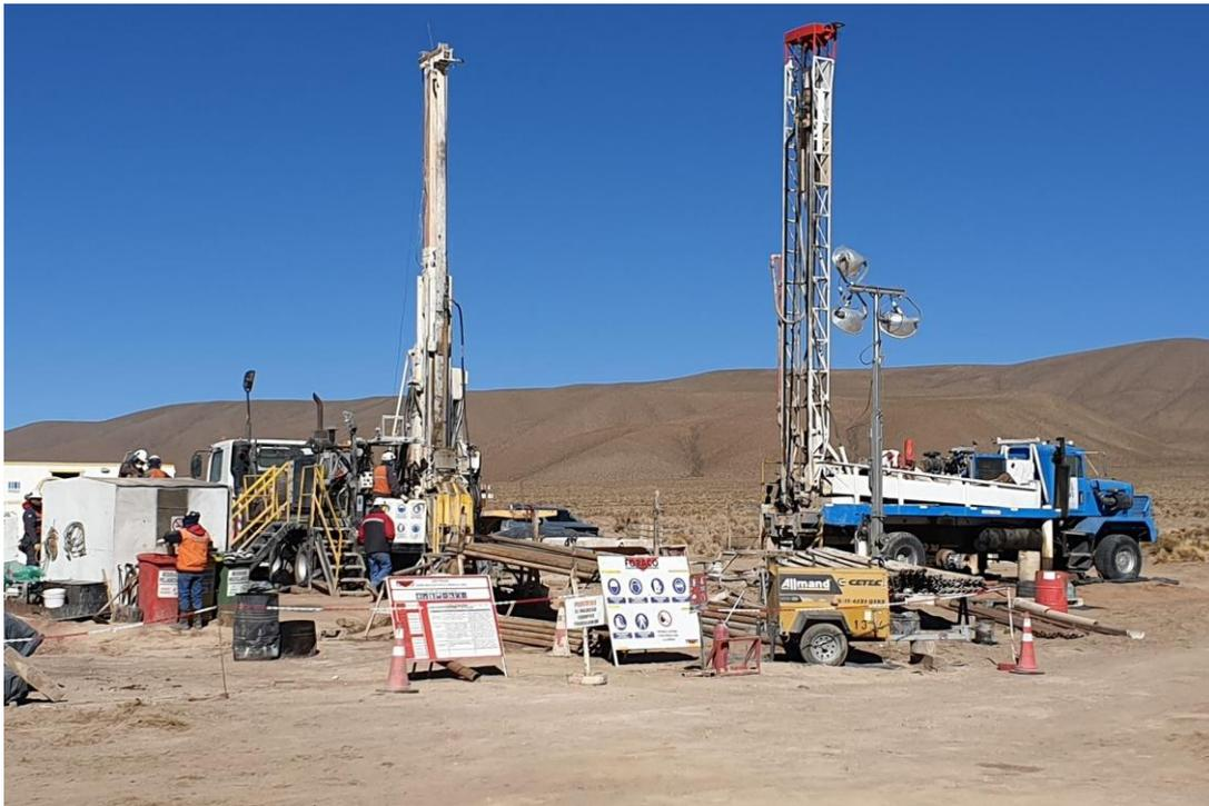
Figure 3: Foraco diamond drill rig (left) and rotary rig at Cauchari.
