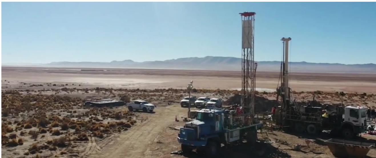
Figure 1: Foraco diamond drill rig (right) and rotary rig at Cauchari overlooking the Cauchari salt lake and development of the adjoining pre-production areas of Ganfeng / Lithium Americas.
