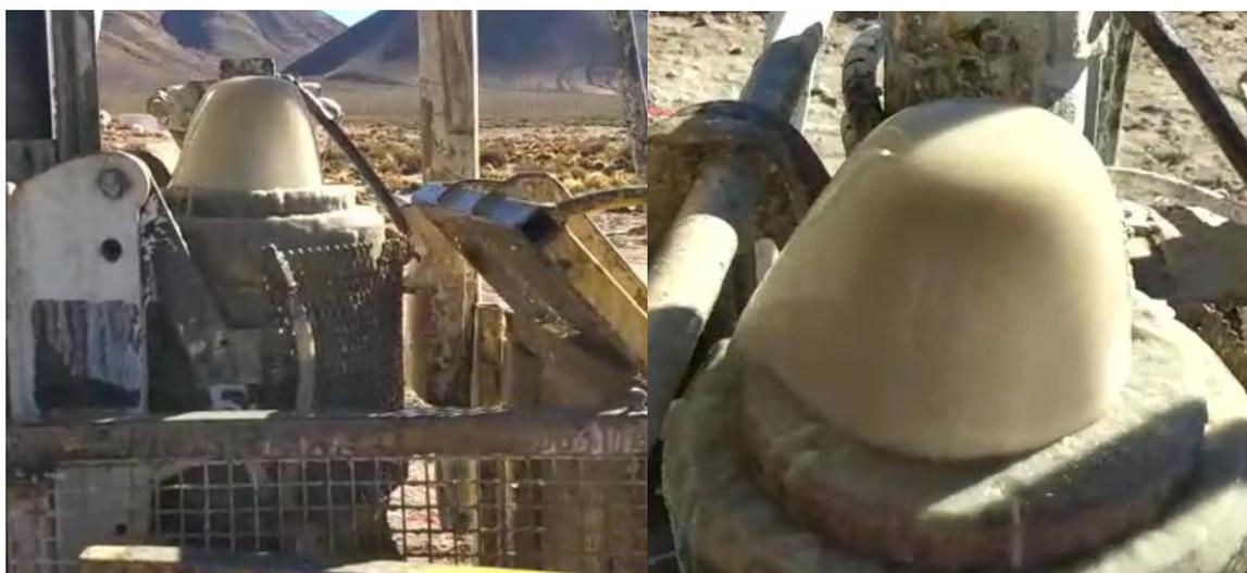
Figure 2: Lithium bearing brines flowing out of the drill head (pale yellow upside down cup shape) from high pressure horizons
