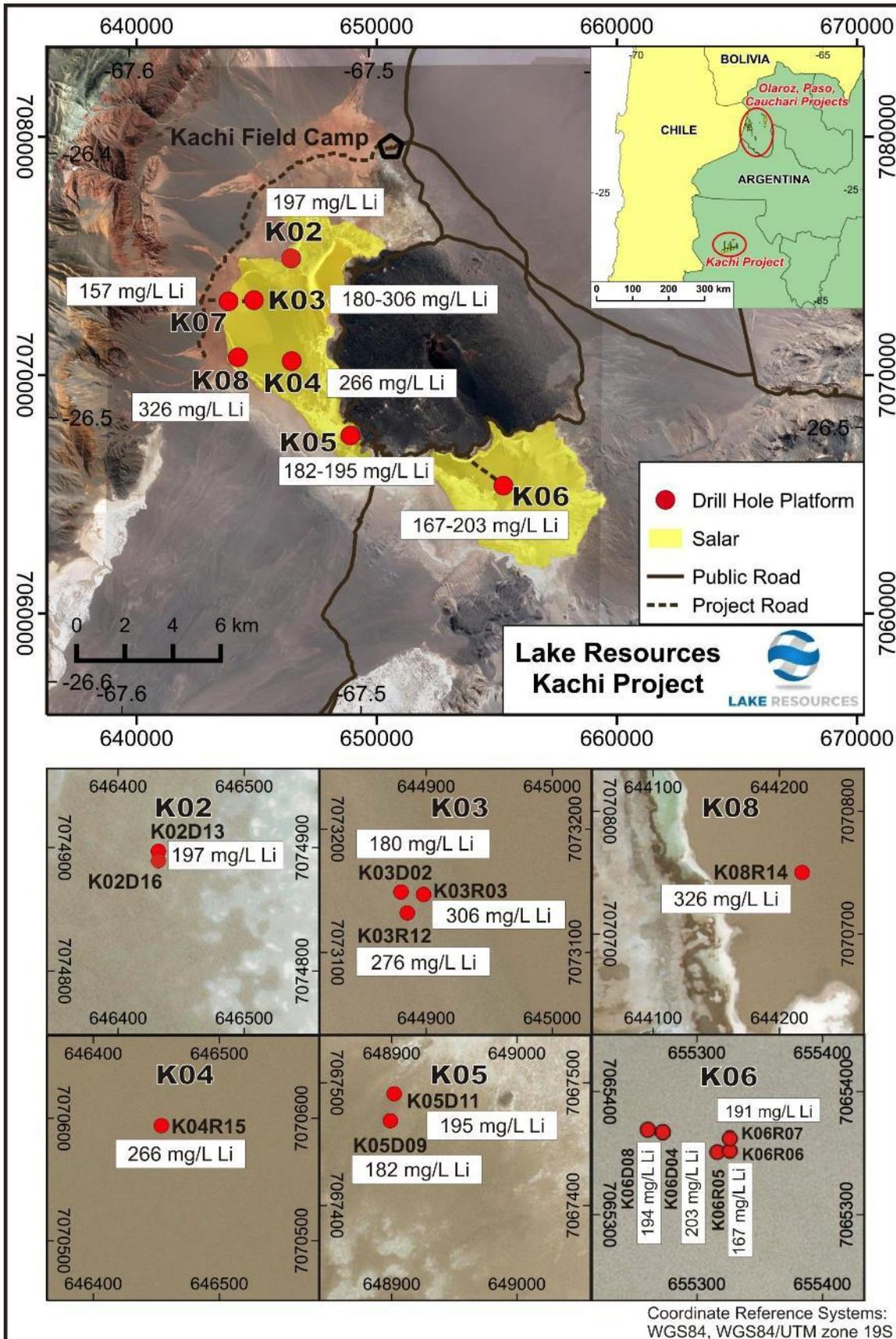
Figure 2. Kachi Lithium Project showing drilling locations, details of the drill hole layout at each location and lithium concentrations for each drill hole which are averaged where multiple brine samples have been taken at various depths.
