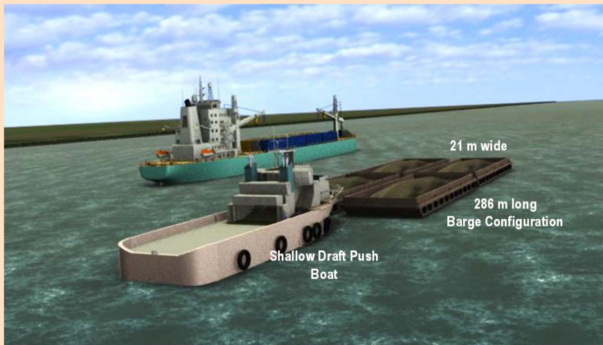
Barge configuration with push boat
