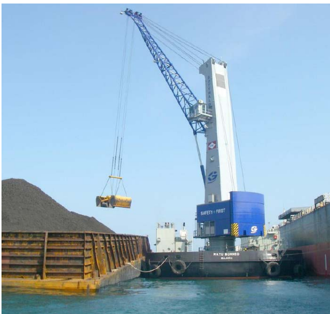
Typical Floating Crane used in Transshipment Operation
