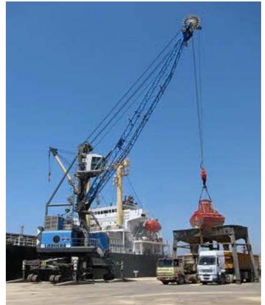
Typical Mobile Harbour Crane with Grab for Barge Unloading
