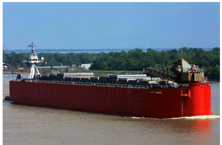
Typical Self Unloading Barges used in Transshipment Operations
