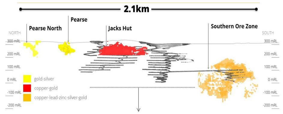
Significant depth potential with only 2% of drilling testing below 350m
