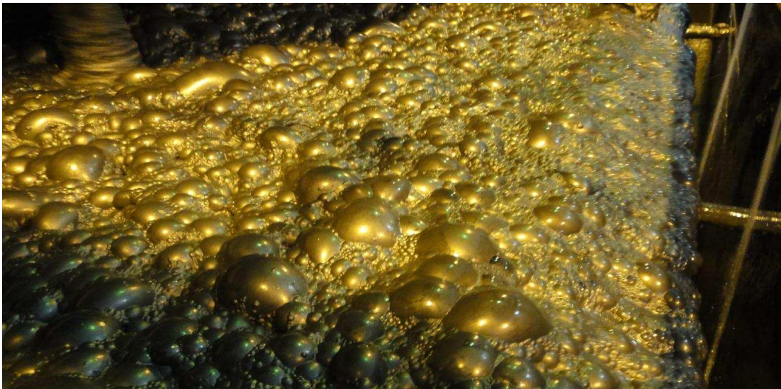
Figure 2: Float Cells with 2.59% copper feed grade on 10 August 2011
