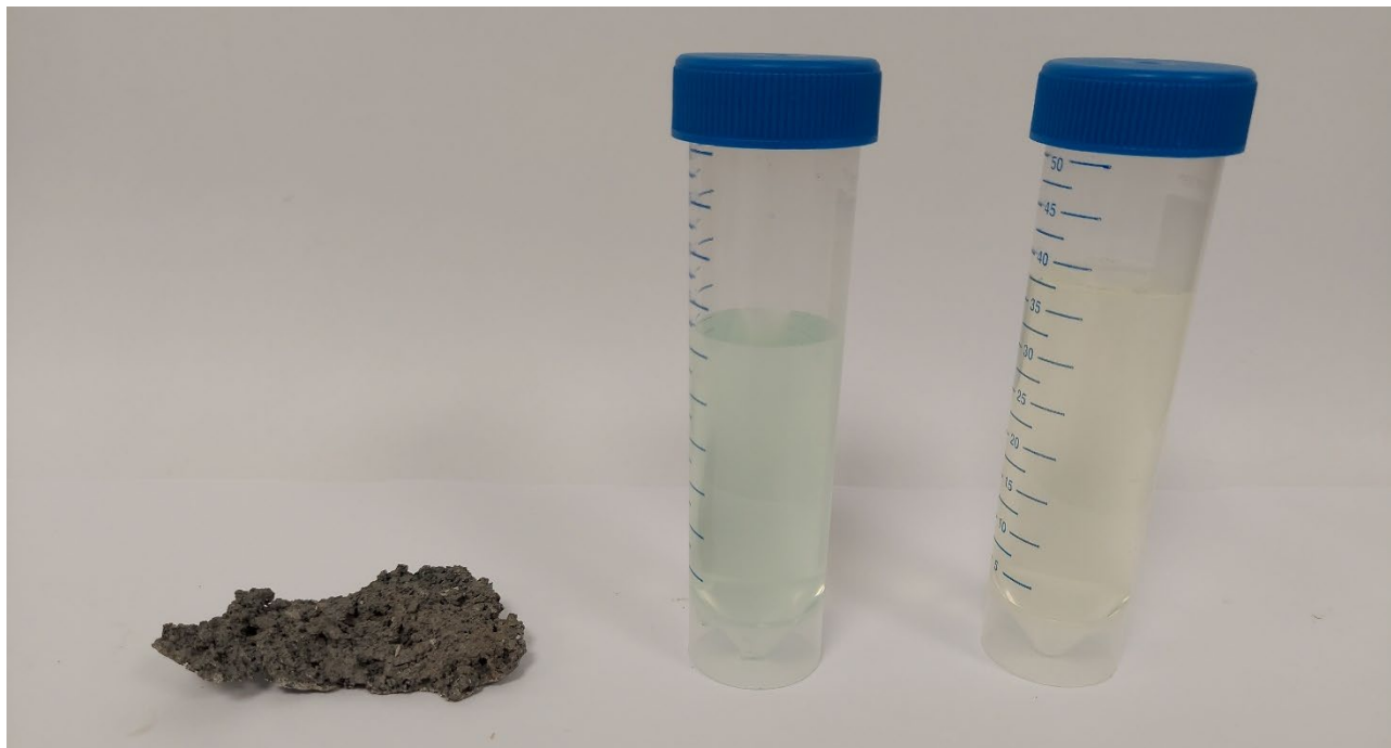
Figure 1: Dysprosium (Dy) and terbium (Tb) alloy feed material (left), and subsequent streams prior to separation to recover high purity (> 99.5%) Dy_2O_3 and Tb_4O_7 products.
