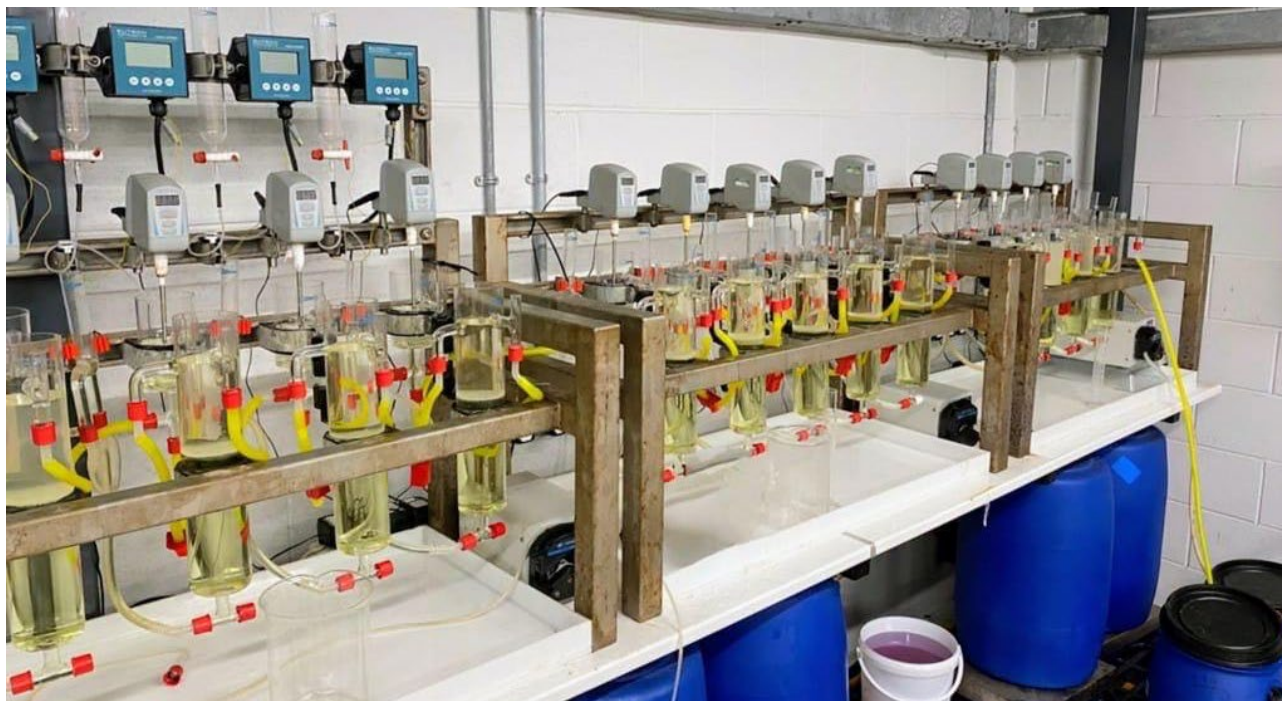
Figure 2: Operating Dy/Tb Separation on the Ionic Technologies Pilot Plant Mixer Settler Circuit at Ionic Technologies' facility in Belfast, UK.
